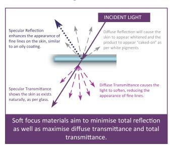
Light can interact with a material in a number of was as shown. Soft focus materials reduce the reflected components of light, which show lines and whiten the skin, and increase the diffuse component of transmitted light softening fine lines. Alusion® enhances the diffusion of light whilst remaining highly transparent, giving a superior more natural look.
